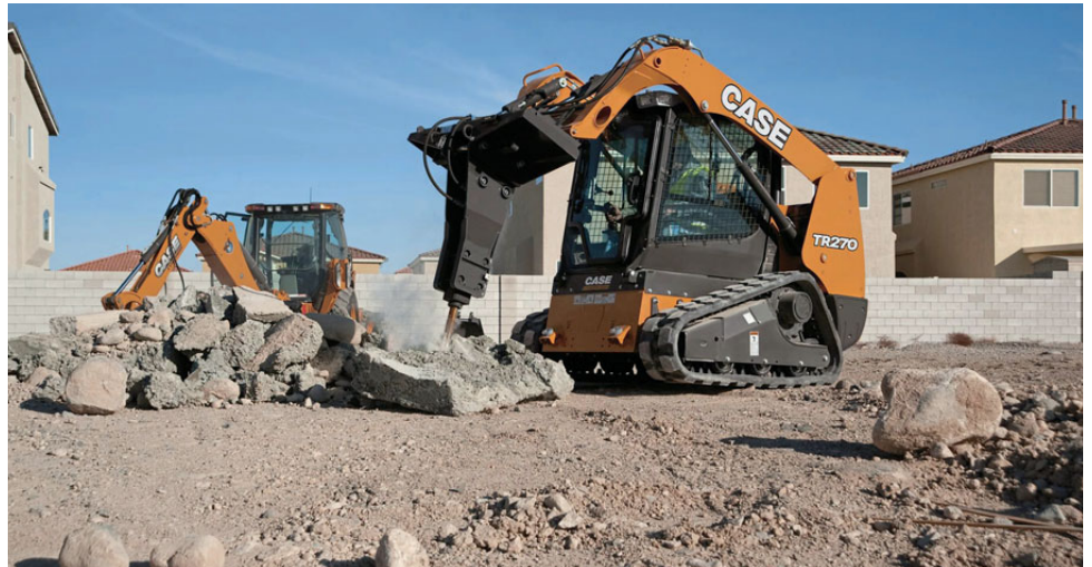
■ Tracked loaders are more suited for working with heavy attachments such as breakers.
