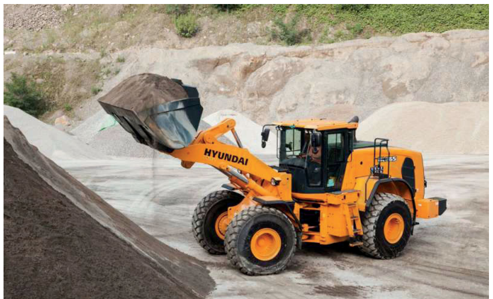
■ A new sound-proofed, air-conditioned cabin is 10% larger than was previously available on older machines.
